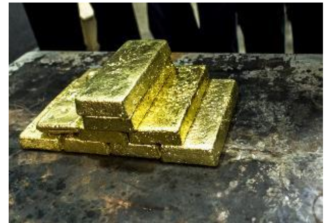
6. Smelting Process to Produce Dore Bar
